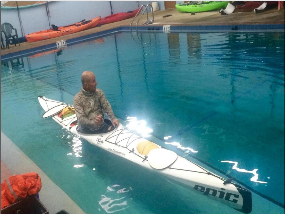
Chief showing the capabilities of a properly loaded kayak. In this demonstration, Chief packed his kayak with a full EC load and spare flotation. He then took the hatches off and purposely flooded the hatches and cockpit to replicate a worst-case scenario situation out on the water. Because Chief's boat was properly packed, it continued to float and could be safely paddled.
